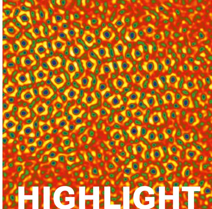
Ultra-high-resolution electron microscopes at the Ernst Ruska-Centre provided unique and fascinating insights into the world of atoms. This microscopic image dating from 2004 shows the metal tantalum with a resolution of 127 picometres. Tantalum is used for metallization in semiconductor electronics.
