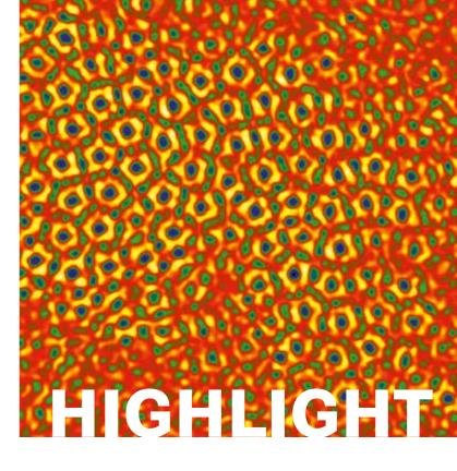
Ultra-high-resolution electron microscopes at the Ernst Ruska-Centre provided unique and fascinating insights into the world of atoms. This microscopic image dating from 2004 shows the metal tantalum with a resolution of 127 picometres. Tantalum is used for metallization in semiconductor electronics.
