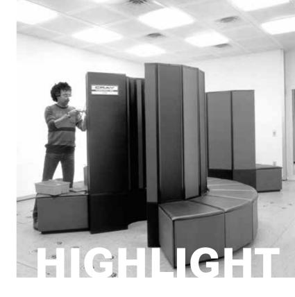
The CRAY X-MP/22 supercomputer was installed in Jülich in 1983. Its 16 megabytes of memory made the computer a sensation.
